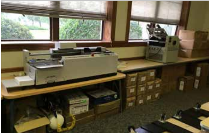
At left under the windows is the DigiBinder for binding paperback books, and to the right is the folder, primarily for folding pamphlets.
